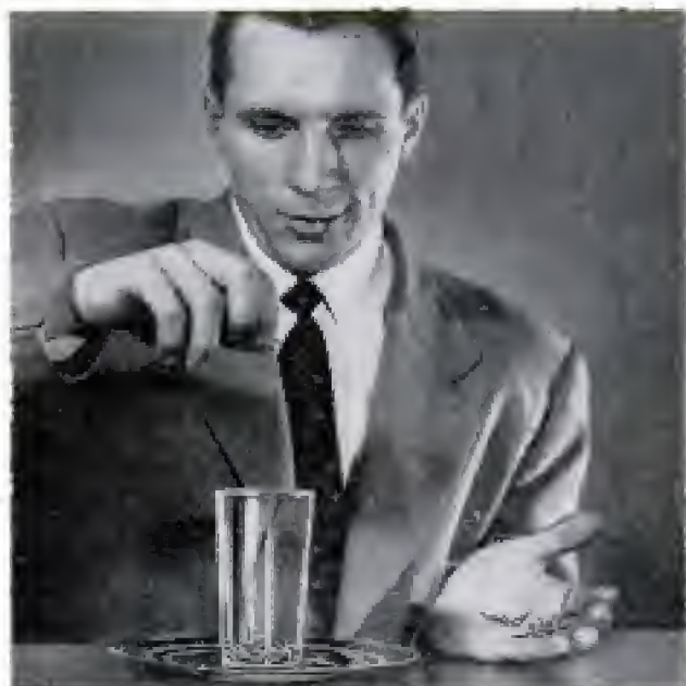
Due to surface tension, water in full tumbler can be displaced to rise above rim without overflowing
